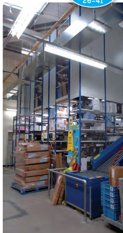
Tiered shelving allows full utilisation of the available ceiling height, with greater storage capacity, which reduces frequent deliveries and increases sales area floor space.
