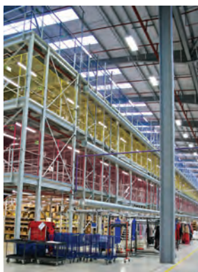
Pick towers can have live storage and garment hanging integrated within the structure, making it a favourite of fashion retail distributors.
