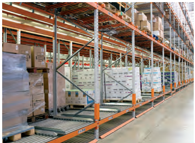
Ideal for perishable and time sensitive products, pallet live storage saves space of up to 60% compared to conventional racking.
